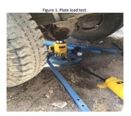
The device was calibrated by national standard organization with coverage factor k=2 correspond to confidence level 95% and the required data were collected after installing equipment, applying load on a steel plate and recording load and settlement rate simultaneously by load and settlement gauges (Barmenkova & Matweeda, 2015).
