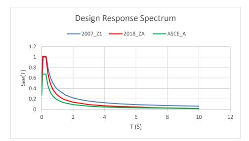
Figure 3. The combined design spectrum curves of the related zone for DD2 seismic ground motion level according to all soil types. Source: Self Elaboration
