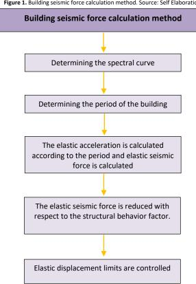
Figure 1. Building seismic force calculation method. Source: Self Elaboration.
