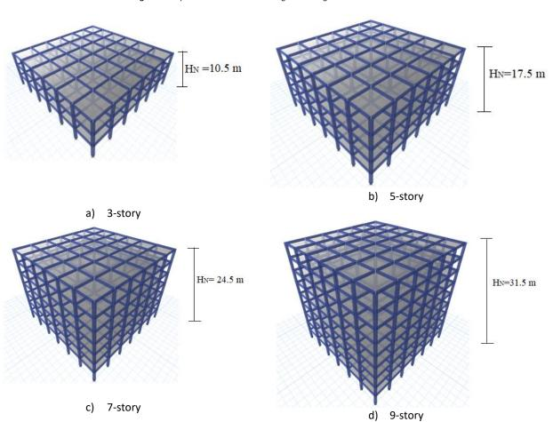
Figure 2. The plan and 3D views for the designed buildings. Source: Self Elaboration.
