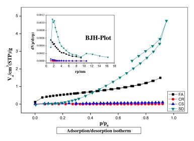
Figure 3. BJH -plot and adsorption/desorption isotherm of ingredients.
