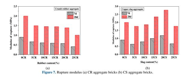
Up to 15%, copper slag substitution shows improved strength than the control mix at the age of 28 days. The maximum strength gains of 46% was obtained in 5% substitution of slag.Fig.8 provides the percentage variation of mechanical properties with the conventional brick mix at the ages of 28 days.
