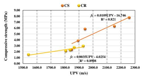
Figure 13. Correlation of UPV and compressive strength of CR and CS aggregate bricks.
