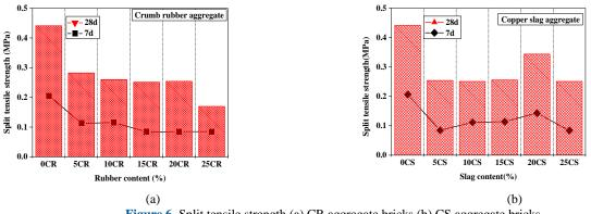
Figure 6. Split tensile strength (a) CR aggregate bricks (b) CS aggregate bricks.
