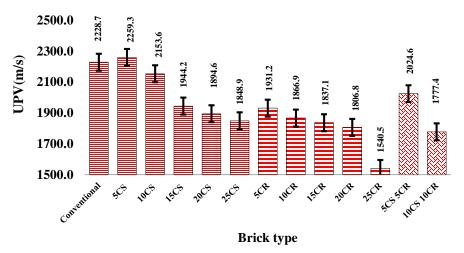
Figure 12. UPV measurements of brick specimens.
