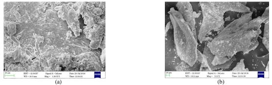
Figure 1. (a) micrograph of rubber aggregate; (b) micrograph of slag aggregate.
