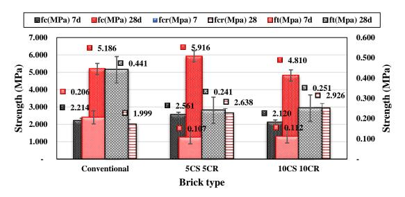
Figure 10. Mechanical properties of combined substitution of CS and CR aggregates.
