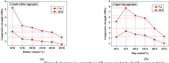
Figure 5. Compressive strength (a) CR aggregate bricks (b) CS aggregate bricks.
