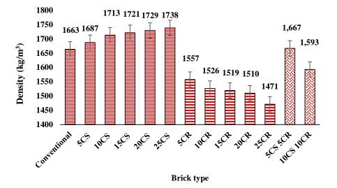
Figure 4. Hardened density of bricks incorporating CR and CS aggregates and its combined substitution.
