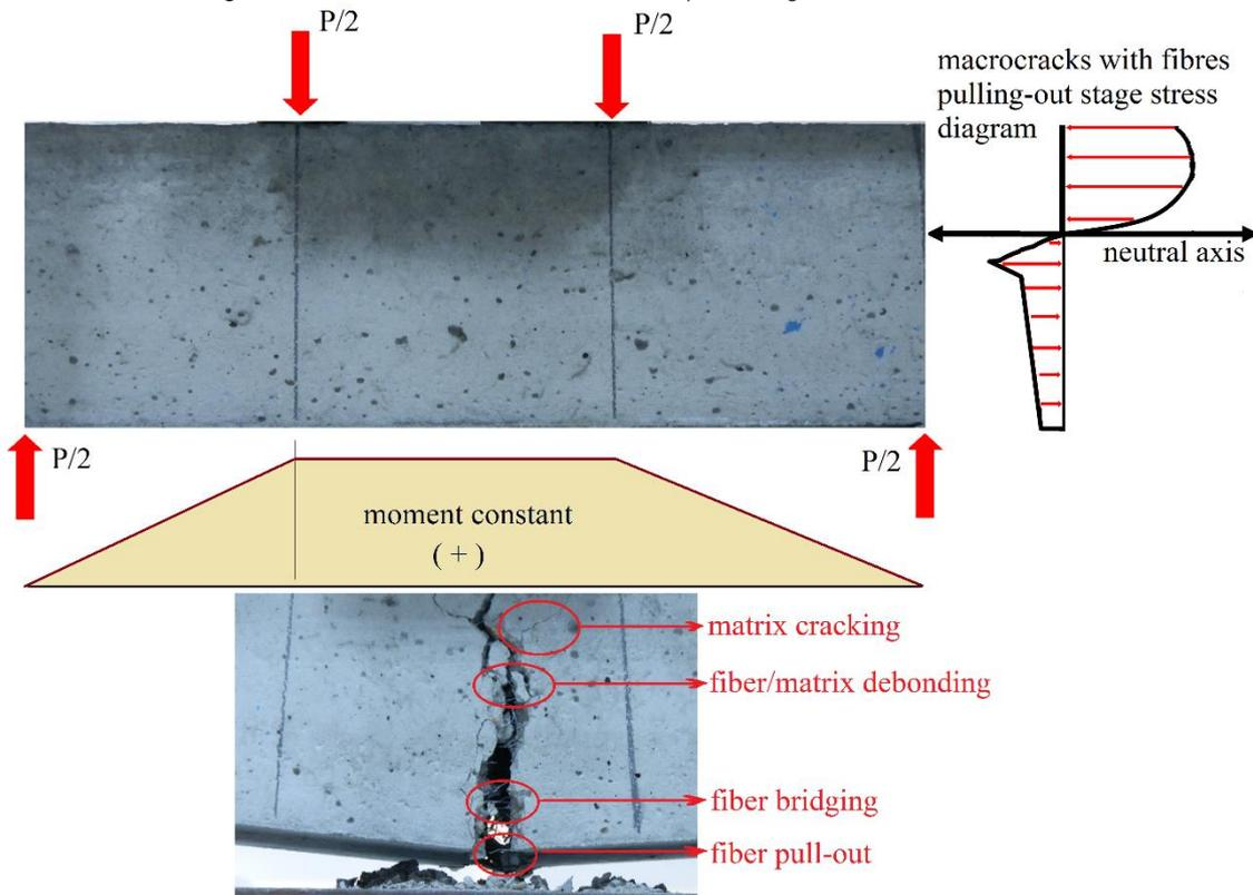
Figure 8. Pulled out fibres on cracked face of the concrete beam specimen. Source: Self Elaboration.
