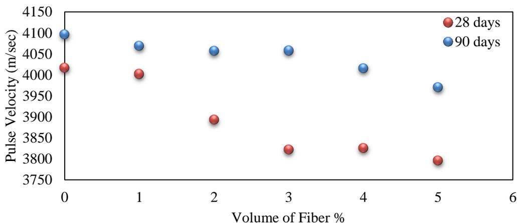
Fiber addition have not improved the UPV of cube samples unlike compressive strength of concrete. The reason is that since self-consolidated concrete were used, increased fiber addition caused more void formation which reduce the workability of the concrete matrix. Therefore, it is assumed that the speed of wave propagation reduces and lower UPV value was ensued.
