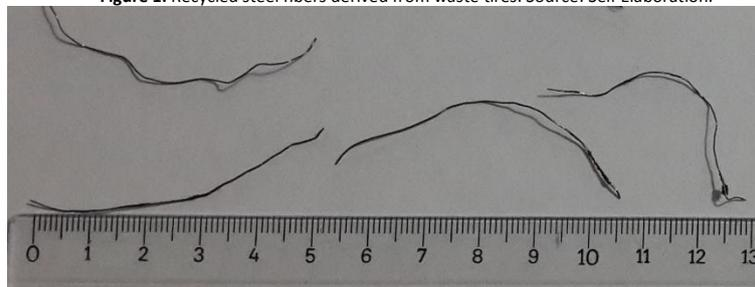
Detailed characterization was performed (Figures 2 and 3) by cleaning steel wires first then measuring the length and diameter of the randomly selected 900 samples of steel wire. It was determined with the micrometer measurement that selected steel wire diameters range from 0.15 to 0.98 mm. Also, as shown in Figure 2, it was determined that the selected steel wire diameters were stacked between 0.22-0.27 mm.
