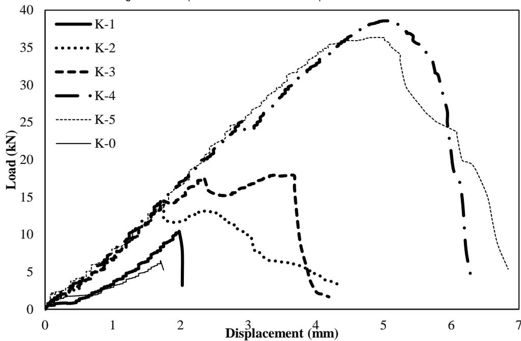
The load-displacement curve of each test sample is given in Figure 6. Figure 6 shows that an improvement in ductility of the samples was observed due to increased fiber ratio. However, after the fiber amount exceeds 4%, reduced strength and reduced energy consumption capacity were observed.
