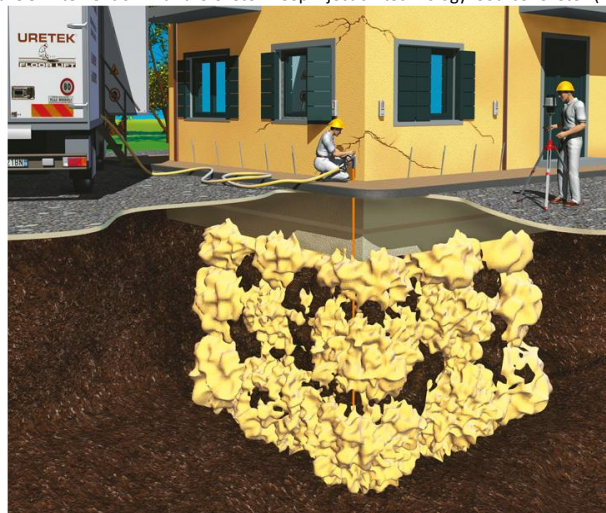
Figure 5. Intervention with the Uretek Deep Injection technology. Source: Uretek (2014).
