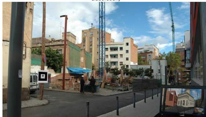
Figure 8. Screenshot of the display with the webcam and the marker AR-Media on the left post and the display of the virtual model in RA in the monitor. (Source: own elaboration)
