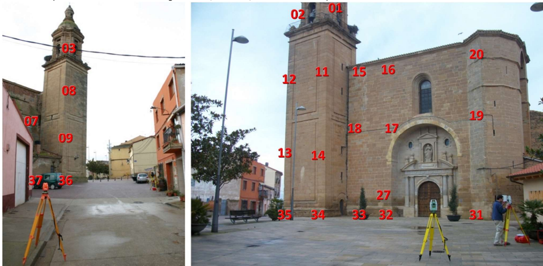
Figure 2. Open spaces around the tower from which the survey observations were carried out. The numbers on the pictures indicate the location and codes of the control points. Total station was arbitrarily set up by resection in eight positions at each epoch, the coordinates of the stationing points were auxiliary and valid only for that specific epoch since the points were not marked on the ground and, therefore, could not be reoccupied. Source: self-elaboration.
