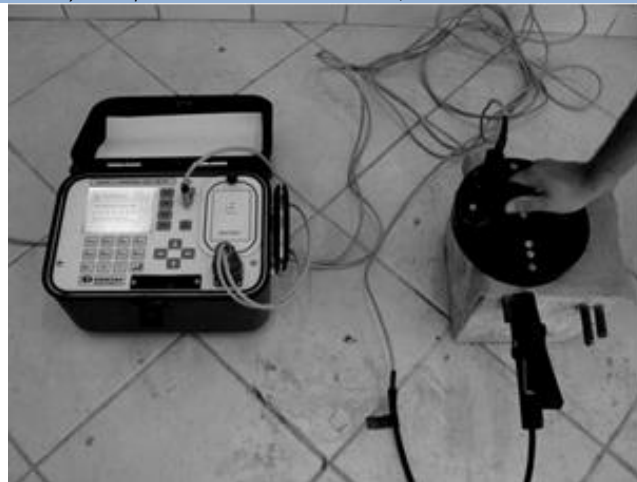
Figure 1. Measurement system used to obtain the corrosion current intensity in the probes. Source: own elaboration, 2010.
