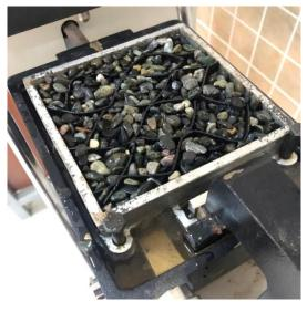
Figure. 2. Geocell placed in shear rings with granular material. (Self-Elaboration).
