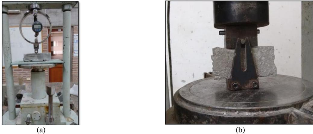
**Figure 5.** (a) flexural strength testing device; (b) compressive strength testing device.
