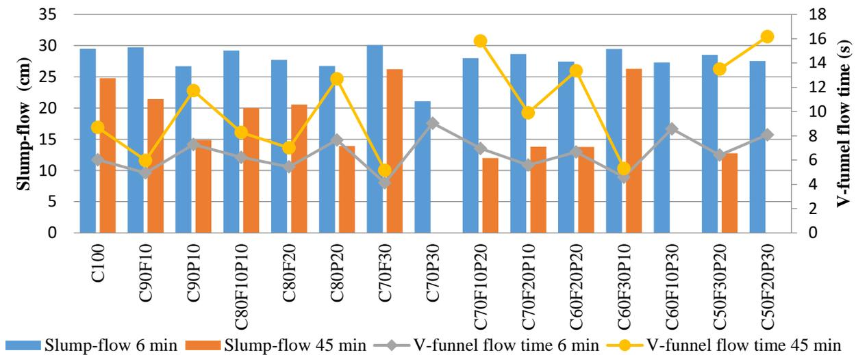
Figure 6. Slump-flow test and V-funnel test results. Source: Self-elaboration.
