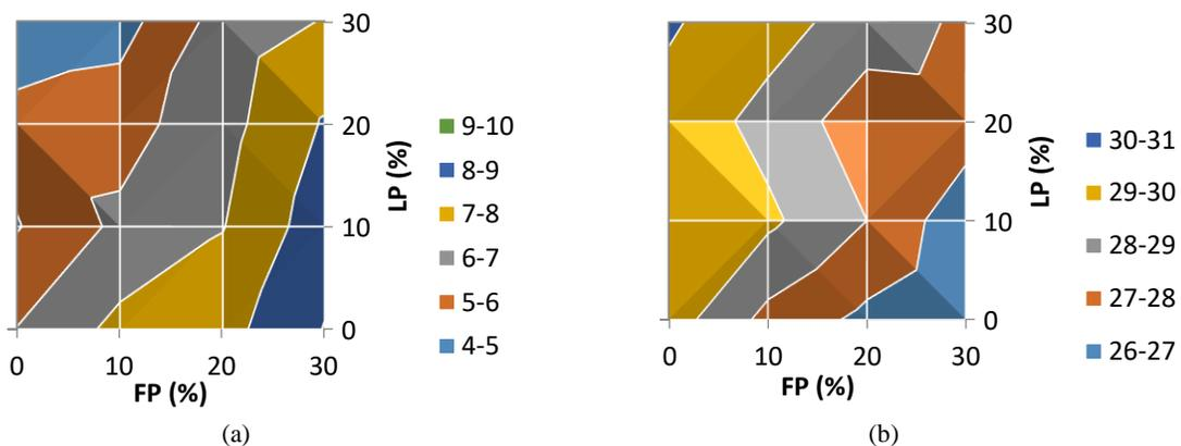
Figure 7. (a) Iso-response curves of V-funnel test results at 6 minutes (s); (b) iso-response curves of slump flow test results at 6 minutes (cm).
