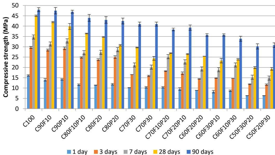
Figure 9. Compressive strength at different ages. Source: Self-elaboration.
