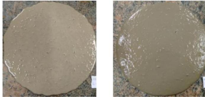
Figure 8. Slump flow tests on mixture with LP (left) and with FP (right).
