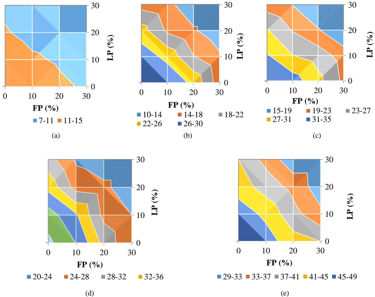
**Figure 10.** Iso-response curves of compressive strength at different ages (MPa); (a) at 1 day; (b) at 3 days; (c) at 7 days; (d) at 28 days; (e) at 90 days.
