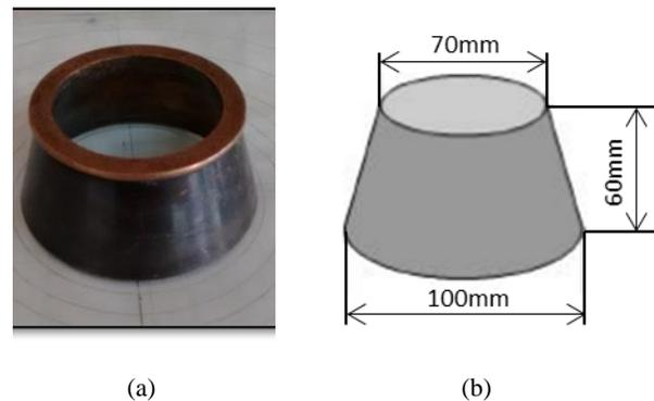
**Figure 4.** (a) Flow cone. Source: Self-elaboration;
