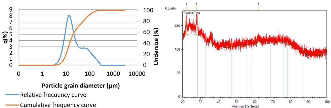
Figure 2. (left) FP grading. (right) FP diffraction pattern.
