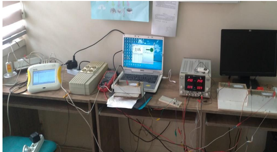
Figure 2. Applying DC to mortars and recording internal temperature values.
