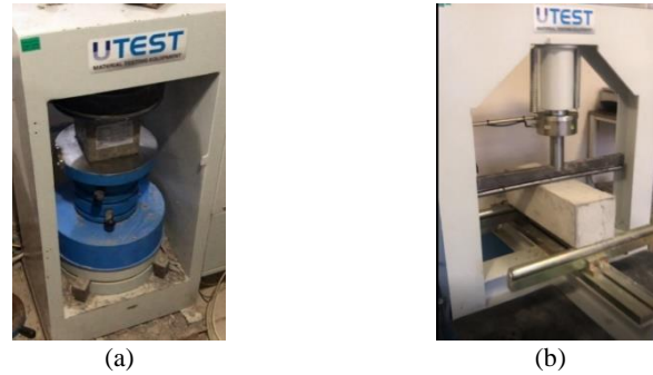
Figure 2. Experimental setup for (a) compressive test on 150x150x150 mm cubic specimens and (b) three-point bending test on 150x150x500 mm prismatic specimens.
