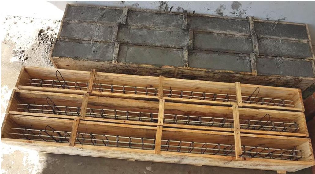
Figure 8. REF beams and GFRP beams assembled before concreting.
