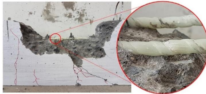
**Figure 11.** Fractured split holder of V1-GFRP.
