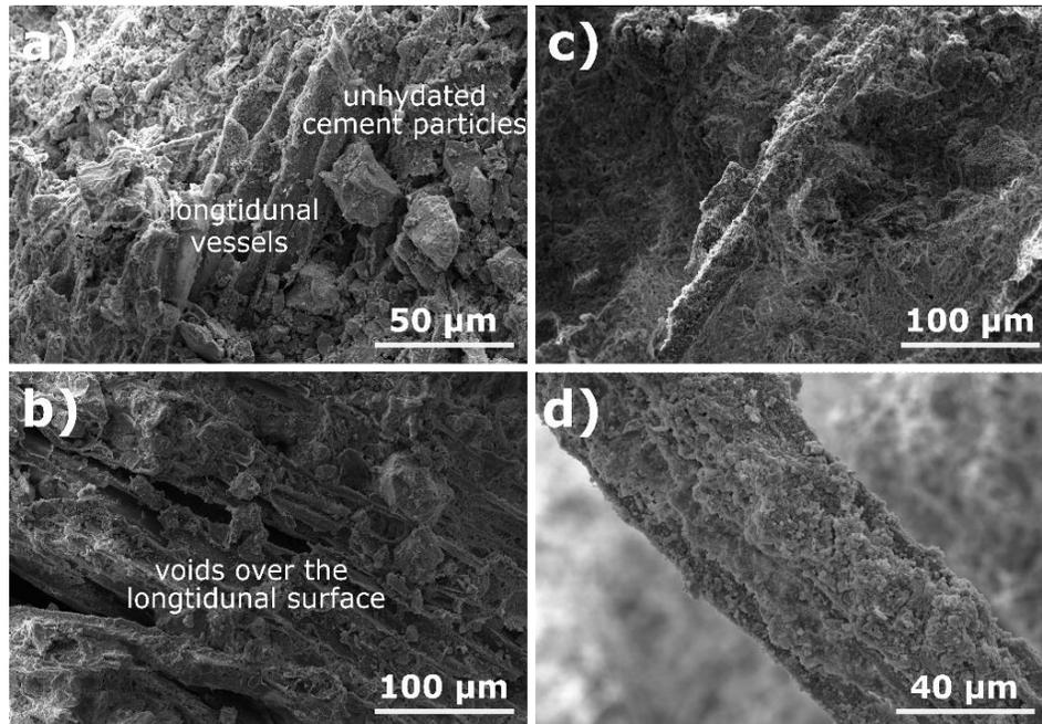
**Figure 7.** SEM images of hemp composites: a) transverse view of a section from Sample 2, b) longitudinal view of a section from Sample 9, c) a general view of section from Sample 11, d) a hemp shiv focused from Sample 12.
