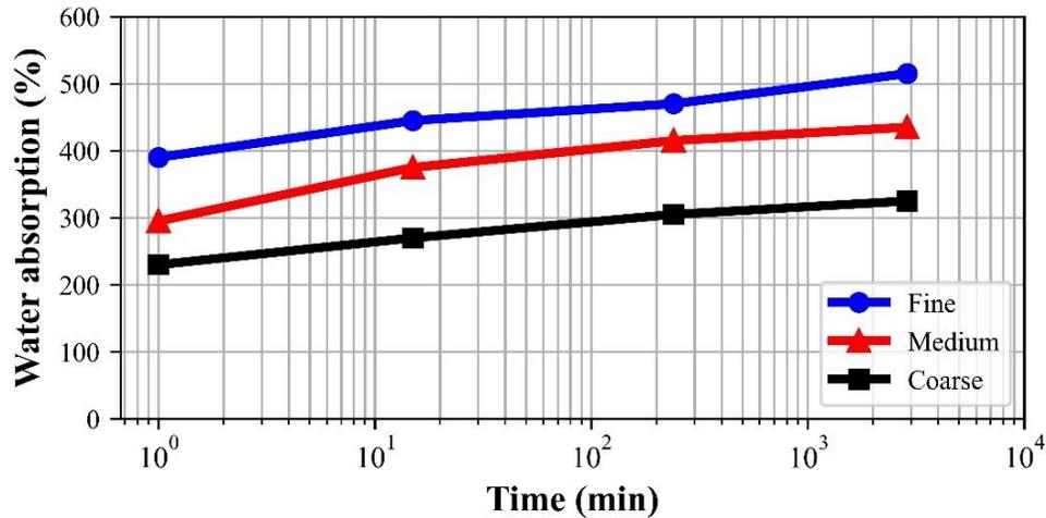
Figure 4. Water absorptions of hemp shiv aggregates used.
