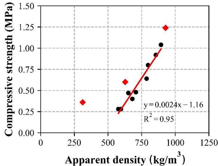
**Figure 9.** Relation between 28-day compressive strengths of samples and apparent density.
