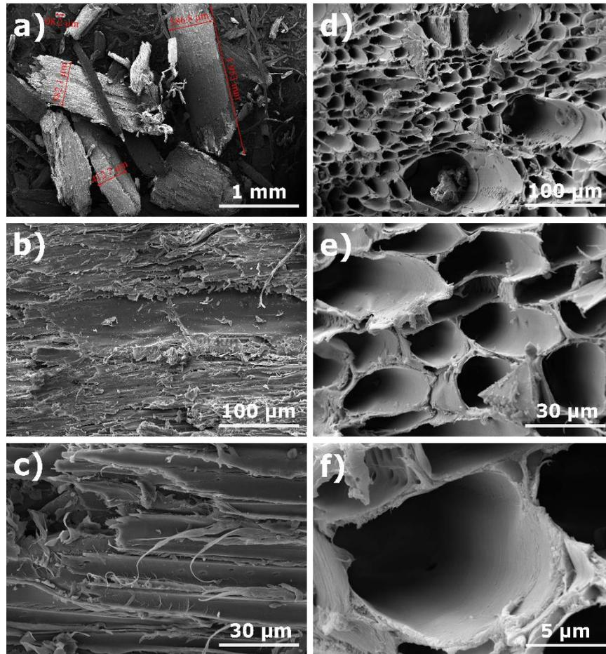
**Figure 5.** SEM images of hemp shiv: a) a macro view of fine hemp shiv aggregates (100x), b and c) longitudinal view of hemp shiv (800x and 400x), d, e and f) cross-sectional view of hemp shiv (1000x, 4000x and 15000x).
