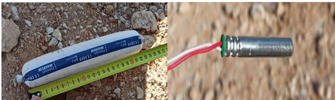
**Figure 10.** Images of the dynamite and the electric detonator used in the tests, respectively.
