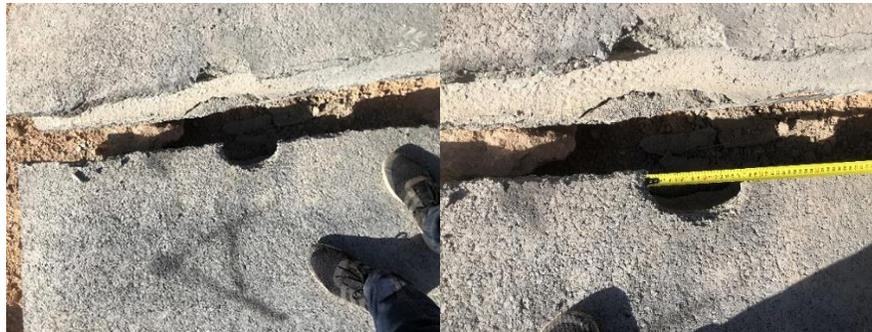
**Figure 11.** Images of supported hollow-core slabs after contact explosions with 500-gr dynamite setups
