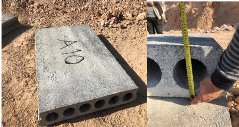
**Figure 9.** Images of hollow-core slabs, hollow-core cross-sections, and prestressing ropes, respectively.
