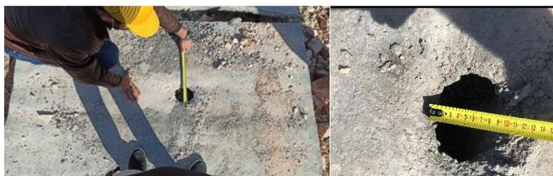
**Figure 15.** Contact explosions of 125-gr explosives on slabs placed on the ground
