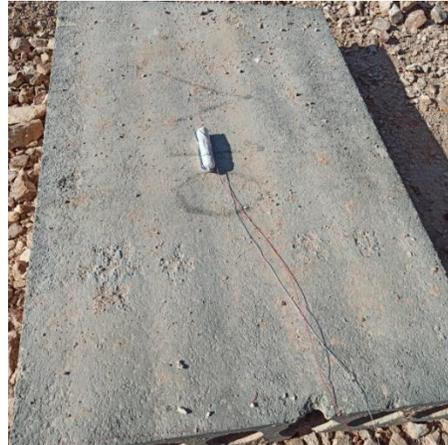
**Figure 13.** Images of the installation of the slabs and the explosives on slabs in the field.
