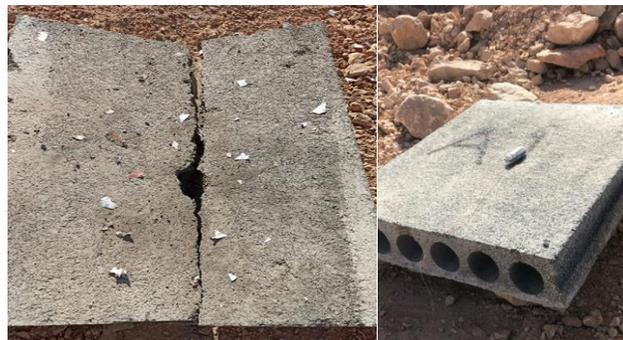
**Figure 12.** Images of supported hollow-core slabs after contact explosions with 250-gr dynamite setups
