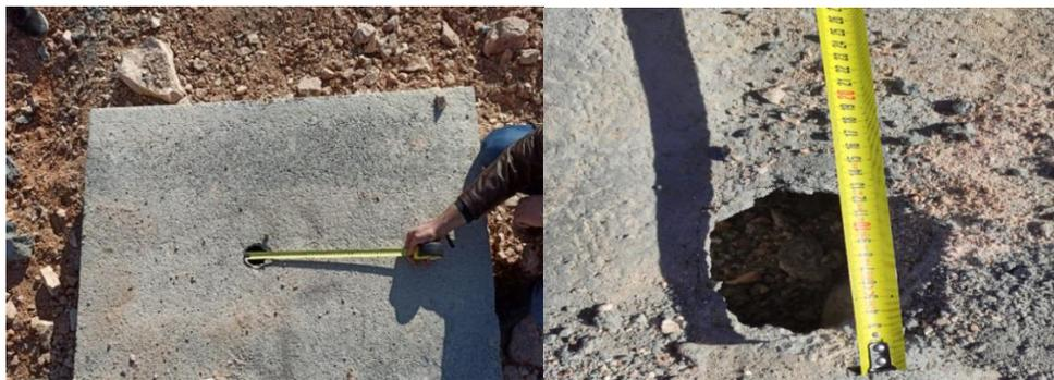
**Figure 14.** Contact explosions of 125-gr explosives on slabs placed on the ground
