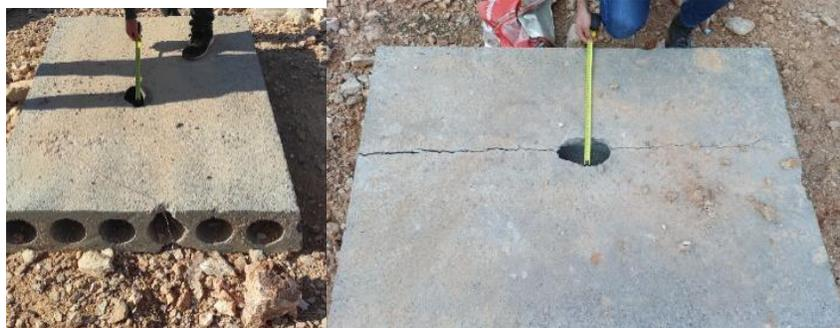
**Figure 16.** Contact explosions of 375-gr explosives on slabs placed on the ground.
