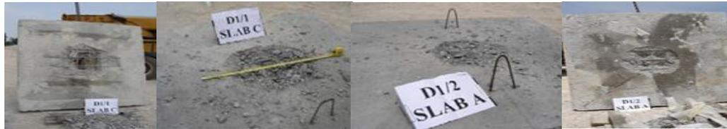
**Figure 1.** Contact explosions and the aftermath of the slabs with 300x300x30 cm dimensions (Wang et al. 2008).
