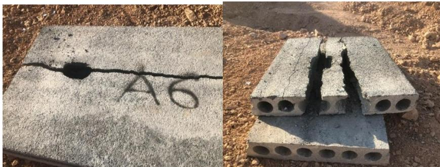
**Figure 17.** Contact explosions of 500-gr explosives on slabs placed on the ground
