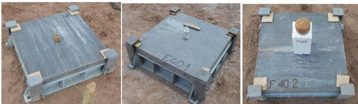
**Figure 5.** Explosion tests on high strength fiber reinforced concrete slabs (Luccioni et al. 2018)
