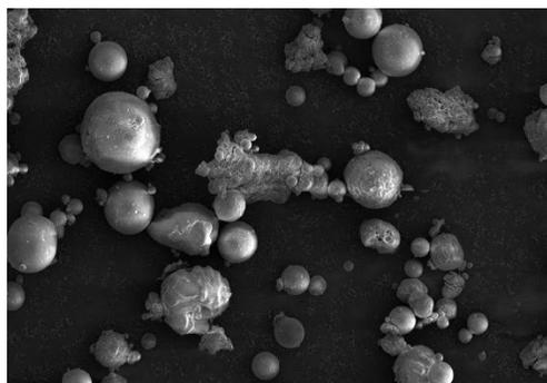
**Figure 1.** SEM image of class C fly ash.
