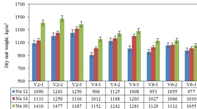
Figure 4. Dry unit weights of the samples.
