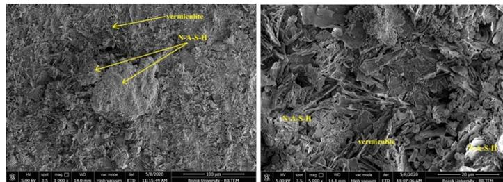
**Figure 15.** SEM images of LGM coded N12V2-3.
