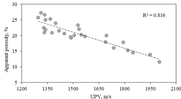
Figure 8. Relationship between apparent porosity and UPV.
