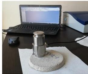
Figure 9. Thermal conductivity test setup.
