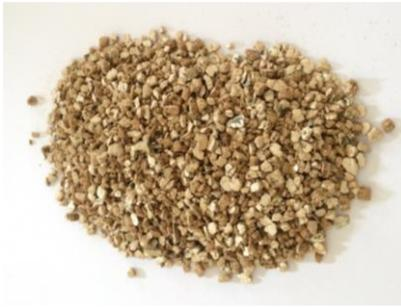
**Figure 2.** Expanded vermiculite used.
