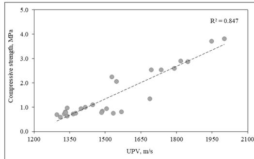
**Figure 13.** Relationship between UPV and compressive strength.
