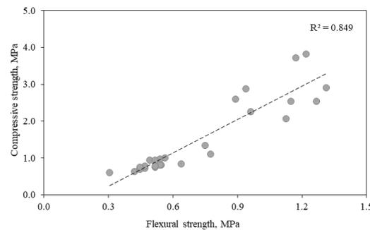
**Figure 14.** Relationship between flexural and compressive strengths.
