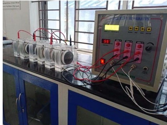
Figure 1. Test setup of rapid chloride permeability of concrete.
