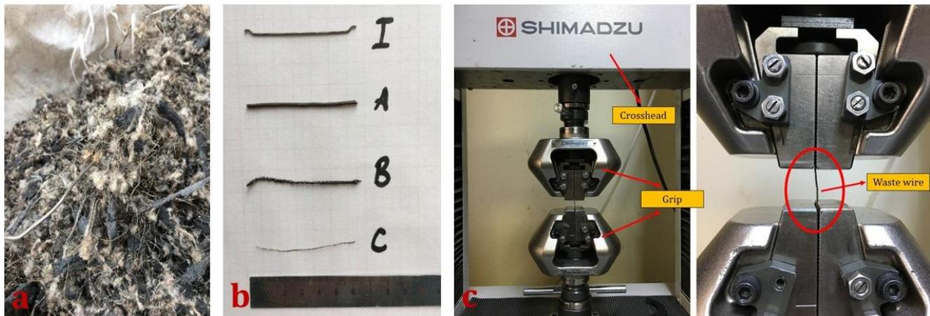
Figure 2. Fibers a) unsorted ELT waste b) types of fibers c) tensile test setup of waste fibers.
