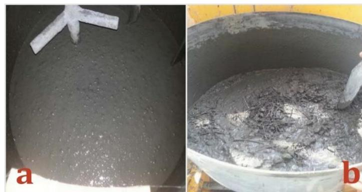
**Figure 3.** (a) Homogeneous mixture and, (b) glomeration.
