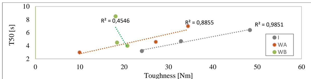
Figure 10. Correlation of fracture toughness and T50.
