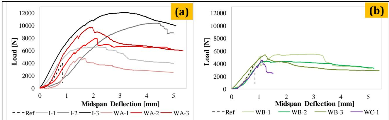
Figure 8. Load-deflection curves (a) Reference, I and WA series (b) Reference, WB and WC series.
