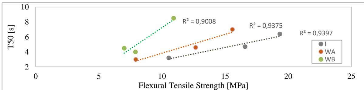
Figure 7. Correlation of flexural tensile strength and T50.
