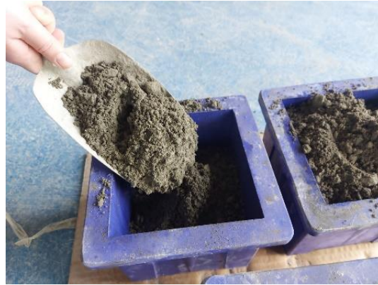
Figure 2. RCC mixture at the fresh state.
