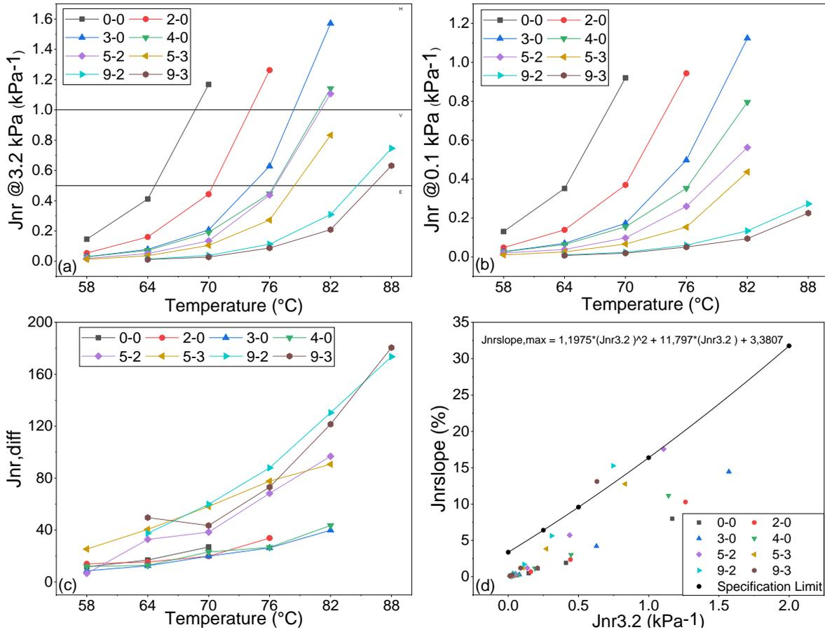
Figure 6. MSCR test results at different temperatures a) Jnr3.2; b) Jnr0.1; c) Jnr,diff; d) Jnrslope.
