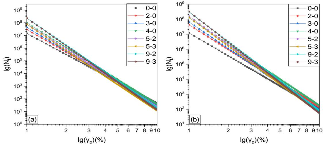
Figure 10. Fatigue lives at different strain levels (a) at 15 °C (b) at 20 °C.
