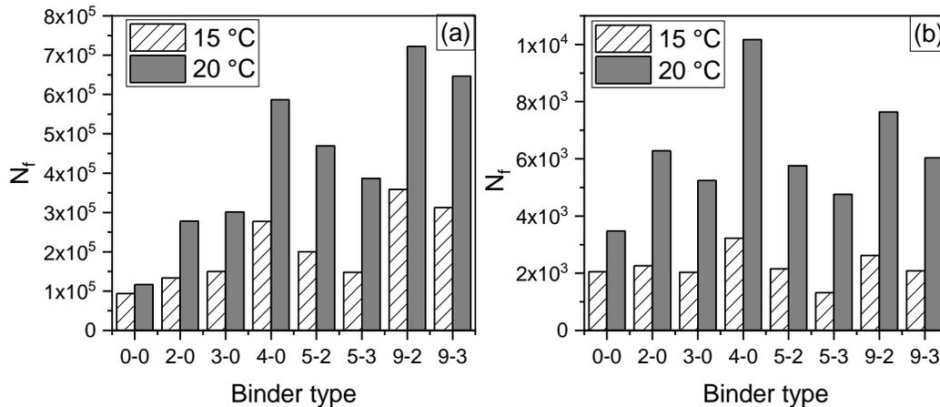
Figure 9. LAS test result: (a) fatigue life at 2.5% strain level and (b) fatigue life at 5% strain level.
