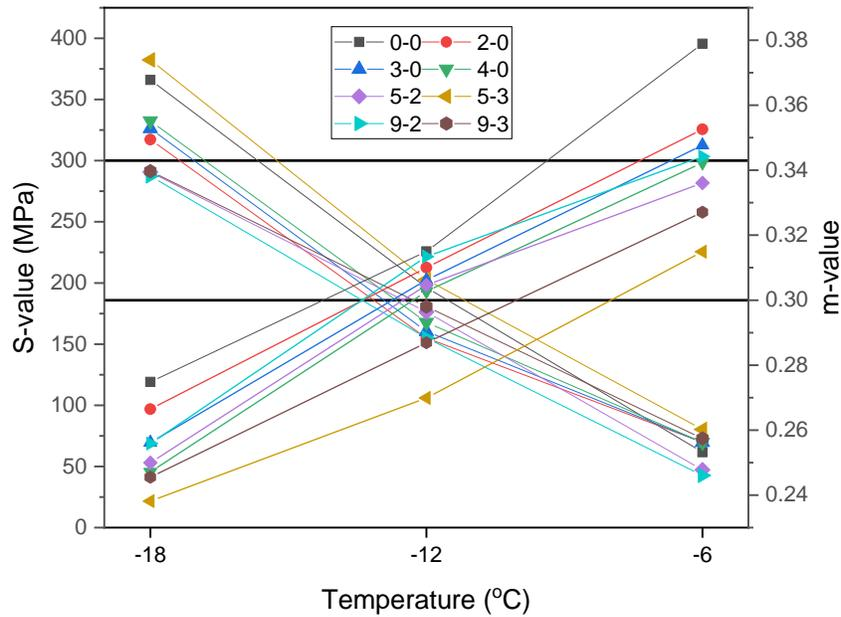
Figure 13. The stiffness and m-value values of pure and modified binders.
