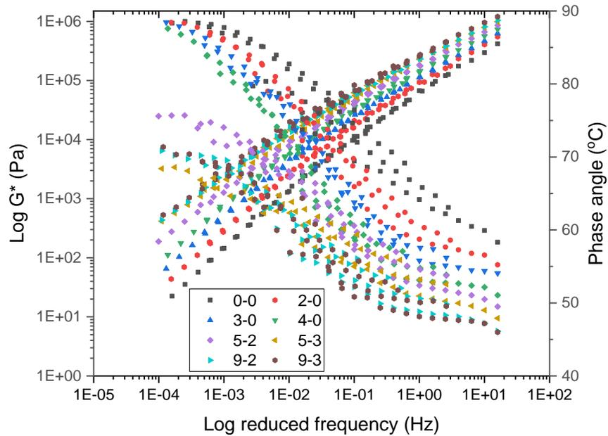
**Figure 2.** Complex module and phase angle master curves of pure and modified binders at 40 °C reference temperature.
