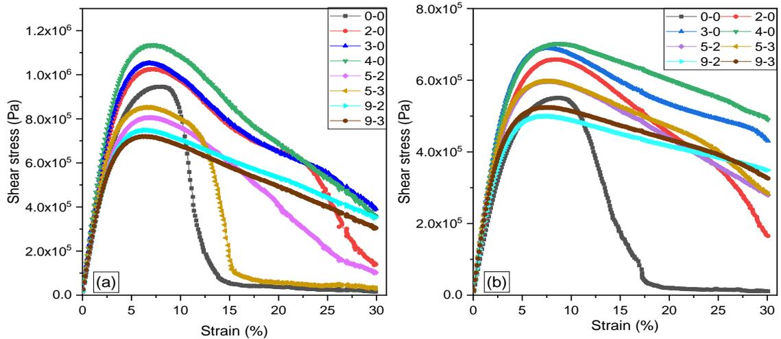
Figure 11. Shear stress versus strain curve of all modified (a) at 15 °C (b) at 20 °C.
