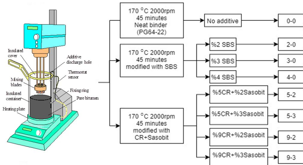
Figure 1. High shear mixer and binder IDs used in the study.
