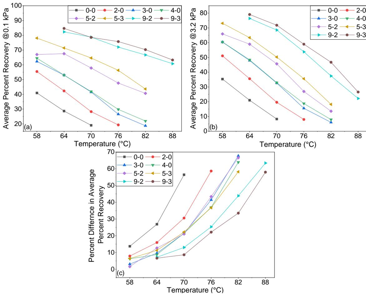
**Figure 7.** MSCR test results at different temperatures a) R3.2 b) R0.1 c) percent difference between averages percent recoveries at 3.2 kPa and 0.1 kPa.
