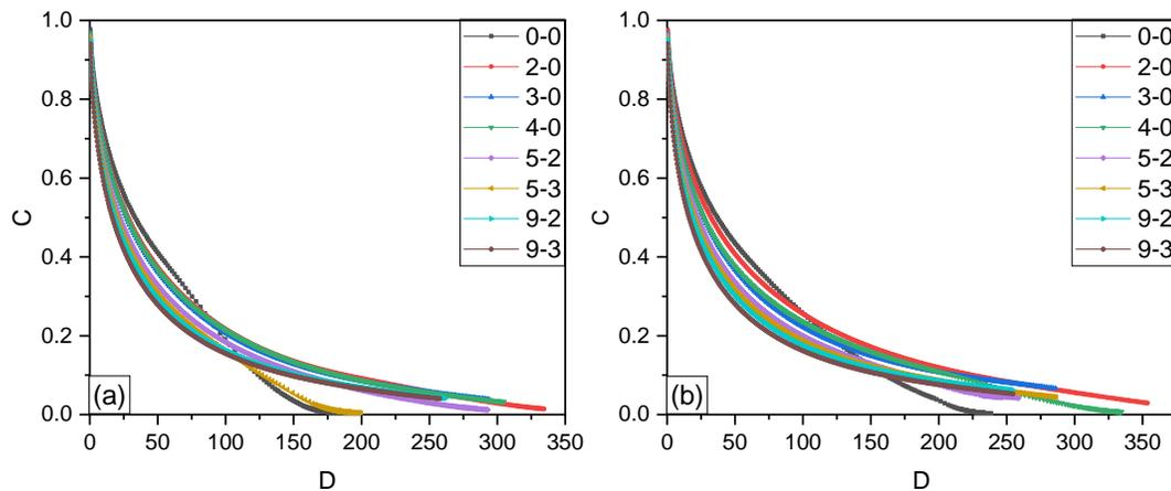
Figure 12. Damage characteristics curves with VECD theory (a) at 15 °C (b) at 20 °C.
