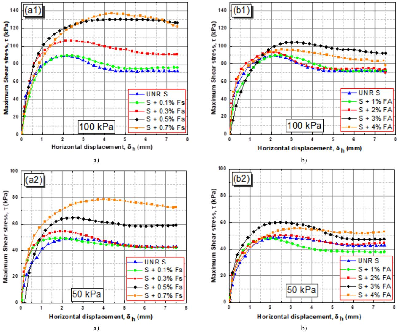
Figure 4. Shear behavior of fiber reinforced sand, shear stress as a function of horizontal displacement, ( $\sigma_N=50$  kPa and  $\sigma_N=100$  kPa);  $D_r=75\%$ : (a) Sisal fiber (Fs), (b) Alfa fiber (FA).
