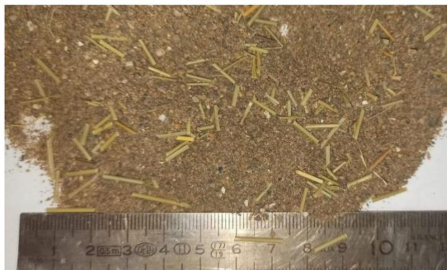
**Figure 2.** Mixture of alfa fiber and sand.
