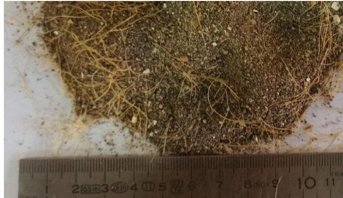
**Figure 3.** Mixture of Sisal fiber and sand.
