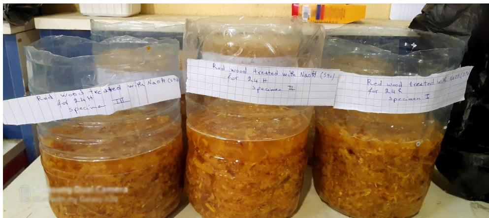
Figure 1. Sawdust treated with NaOH.
