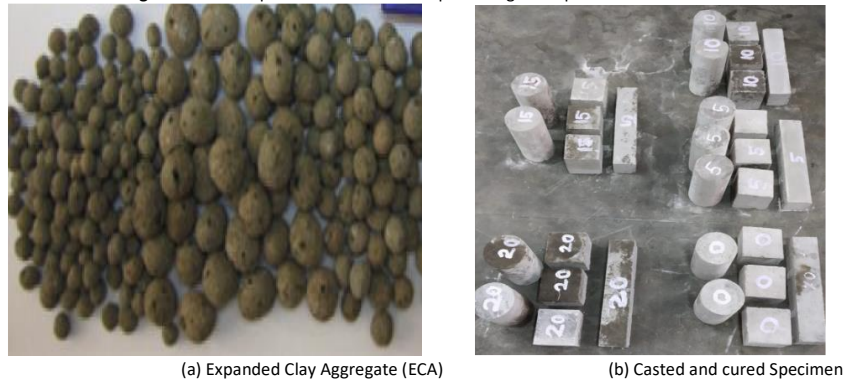
Figure 1. Casted specimen with different percentage of replacement of ECA.
