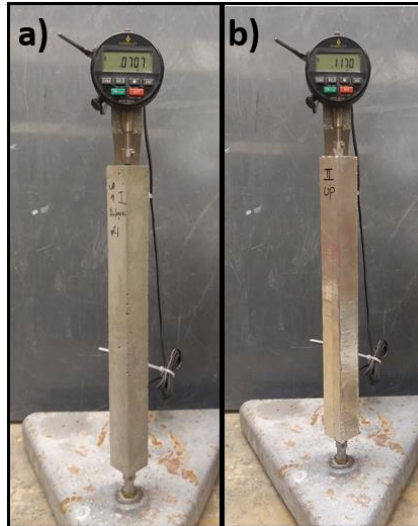
Figure 3. Shrinkage test prisms for ASTM C157. a) Unsealed sample and b) sealed sample with aluminum tape. (Source: authors).
