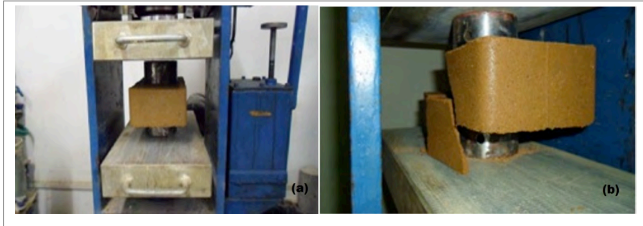
Figure 4. Rupture of the blocks
