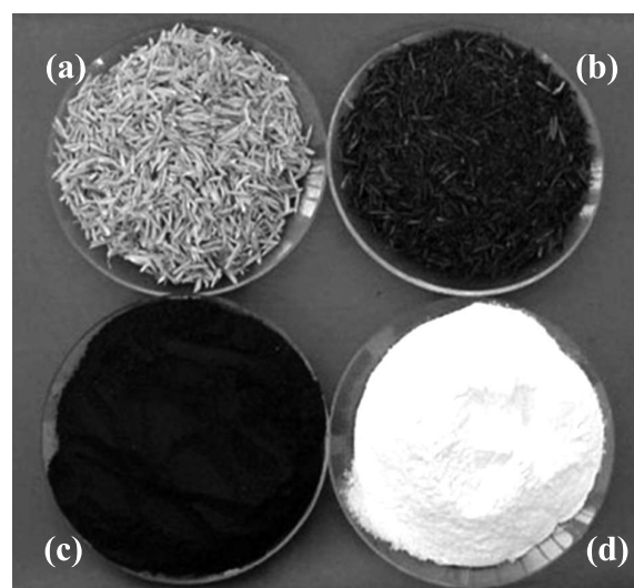
Figure 1. Phases of silica from rice husk production: rice husk (a), rice husk ash before (b) and after (c) of grinding and silica from rice husk (d)
