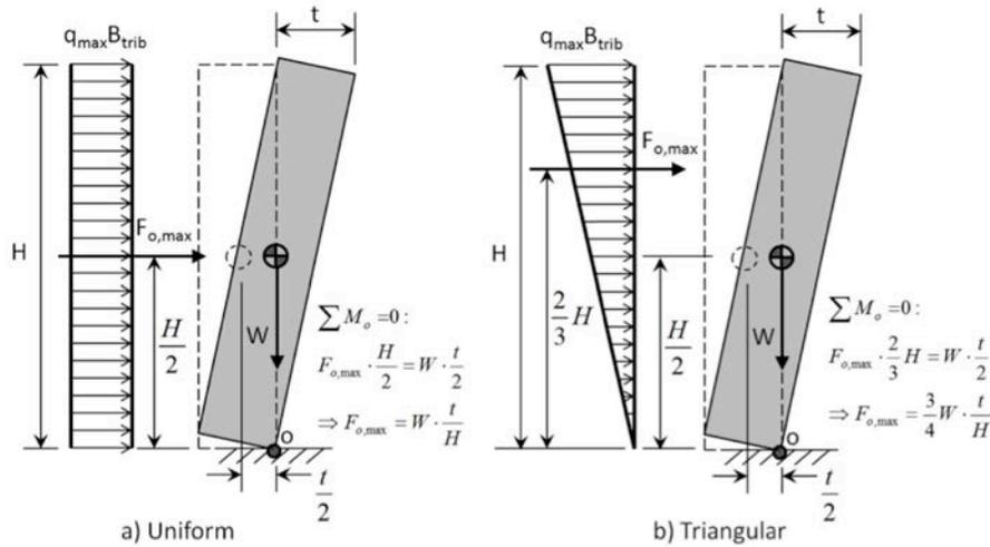
Figure 6. Rigid Cantilever wall at incipient rocking
