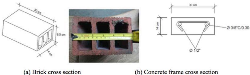
Figure 4. Masonry and concrete frame dimensions and reinforcement.
