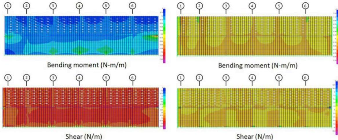
**Figure 11.** FE model force results under uniform wind pressure
