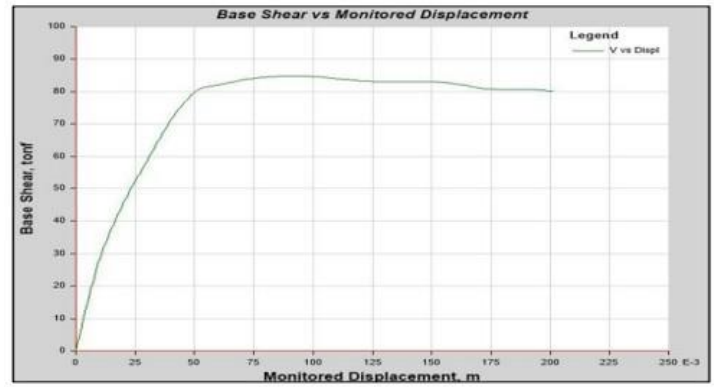
Figure 18. Base shear vs displacement – Block I. Note: Own Elaboration
